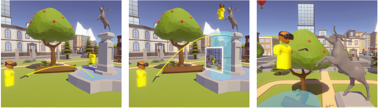
Fig. 1: Teleportation to a mid-air target using our Simultaneous or Two-Step technique. Left: Conventional target specification for teleportation using a selection parabola. A preview avatar shows the future position in the environment. Middle: Simultaneous allows to specify the new elevation with the controller’s touchpad while moving the parabola. Two-Step allows the user to select a reference position on the same elevation before tilting the controller to move the preview up or down. For both techniques, a portal window shows the preview avatar at the new elevation. Right: Once confirmed, the user is teleported to the specified position.
