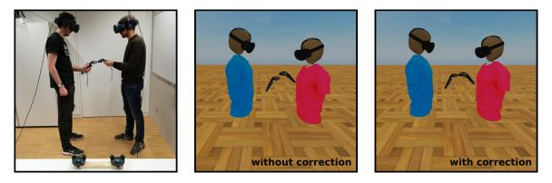
Figure 1: Two collocated users wearing *HTC Vive* displays interact with a shared collaborative virtual environment (left). Without additional mechanisms, both users are tracked and represented in slightly different coordinate systems (middle). We present a procedure for mapping the tracking data to a common coordinate system to allow for spatially consistent interactions (right).
