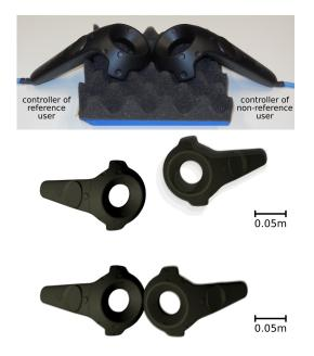
Figure 2: Hardware setup of our experiment (top) and overlaid top views of the 15 controller visualizations in the virtual environment without (middle) and with (bottom) our correction computations activated.
